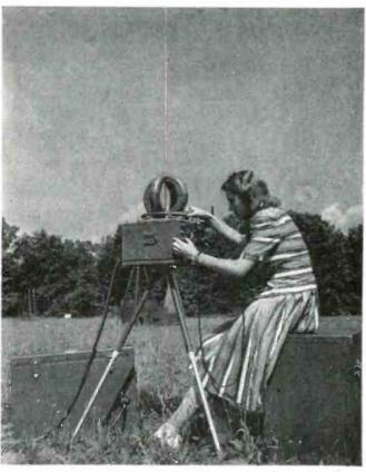
A feminine worker at the Signal Corps Development Lab, checking meteorological equipment. Note double loops.
