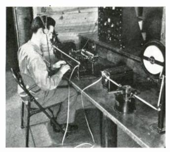
Operator reading automatic tape of high-speed radio transmission. Coordination is essential to efficiency.
