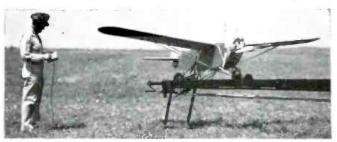
A small radio-controlled glider was developed for target purposes during the period between the two world wars.
