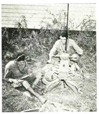
Designed for field use—this pack set is transported on mule or borseback. Hand-driven generator supplies power.
