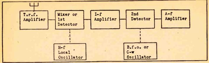
Block diagrams are used to show sequence of circuits. This one represents a superheterodyne receiver.
