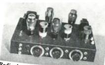
Radiophone Kit—complete RF modulator and power supply on one chassis. For instructions in maintenance and tuning, Can be keyed for code work.
