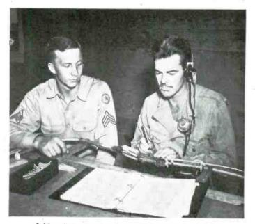
Cable-splicing student, testing a large cable with the aid of bridge—familiar to all Signal Corps men.
