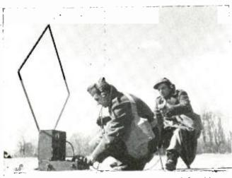
Compact, self-powered field set is operated by this two-man team. This set uses a square loop antenna.
