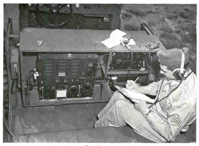
Interior of scout car. The small compartment above the receiver holds a spare set of all tubes required for the radio equipment.
