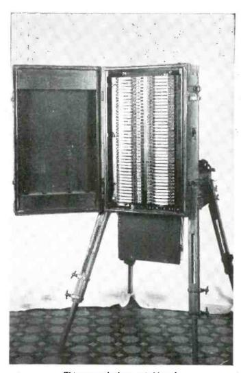
This camp telephone switchboard, used widely in 1915, is very crude compared to new equipment.
