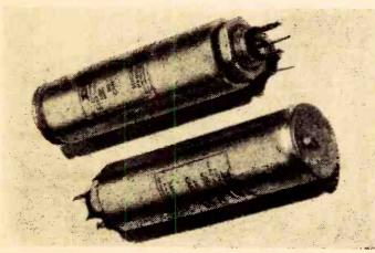
Wet type electrolytic condensers—used in receivers.
