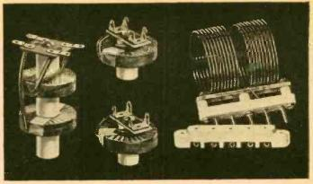
RF chokes and low-power transmitter inductance coil.
