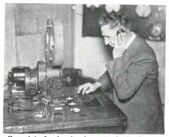
Heart of the Sound studio—the monitor booth. Operator controls volume of sound as it is photographed onto film.
