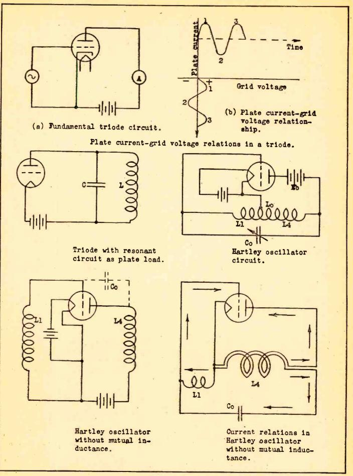
You will study many oscillator circuits. Several are shown in this schematic diagram.
