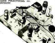
Build this SUPER-HETERODYNE CIRCUIT containing a preselector, oscillator-mixer-first
