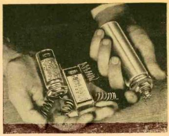
Three types of electrolytic filter condensers.
