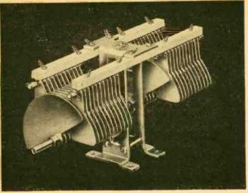
Balanced two-gang variable transmitting condenser.
