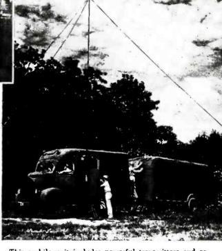
This mobile unit includes powerful transmitters and receivers (in trailer unit). Truck contains generators.
